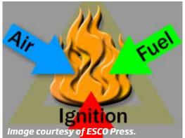
« Figure 1 The combustion triangle consists of three requirements that react fuel, oxygen and heat (or ignition source) to produce heat.
